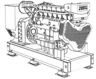
6-cylinder, 4-stroke, direct-injected, and turbo-charged marine diesel engine.
